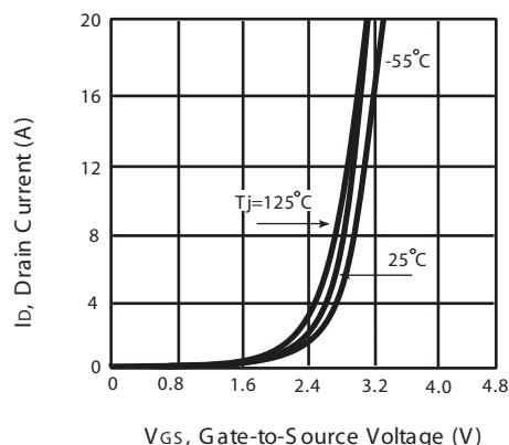
Figure 2. Transfer Characteristics
