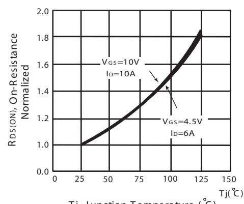
Figure 4. On-Resistance Variation with Drain Current and Temperature
