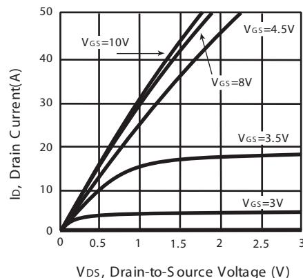
Figure 1. Output Characteristics
