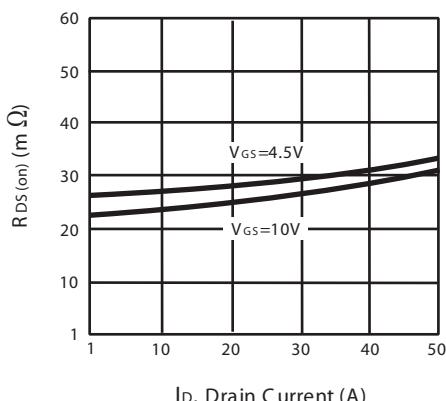
Figure 3. On-Resistance vs. Drain Current and Gate Voltage
