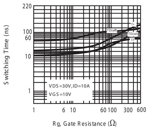
Figure 11. switching characteristics
