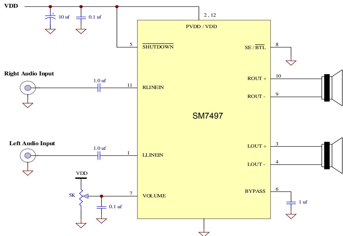
Figure 1. Typical Bridge-Tied-Load(BTL) audio amplifier application circuit for an LCD monitor
