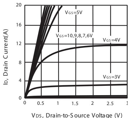
Figure 1. Output Characteristics
