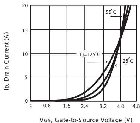
Figure 2. Transfer Characteristics
