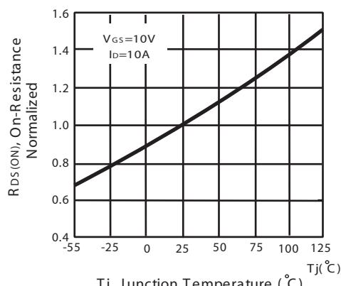
Figure 4. On-Resistance Variation with Drain Current and Temperature
