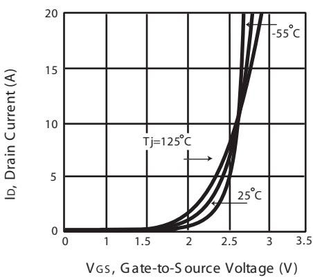
Figure 2. Transfer Characteristics
